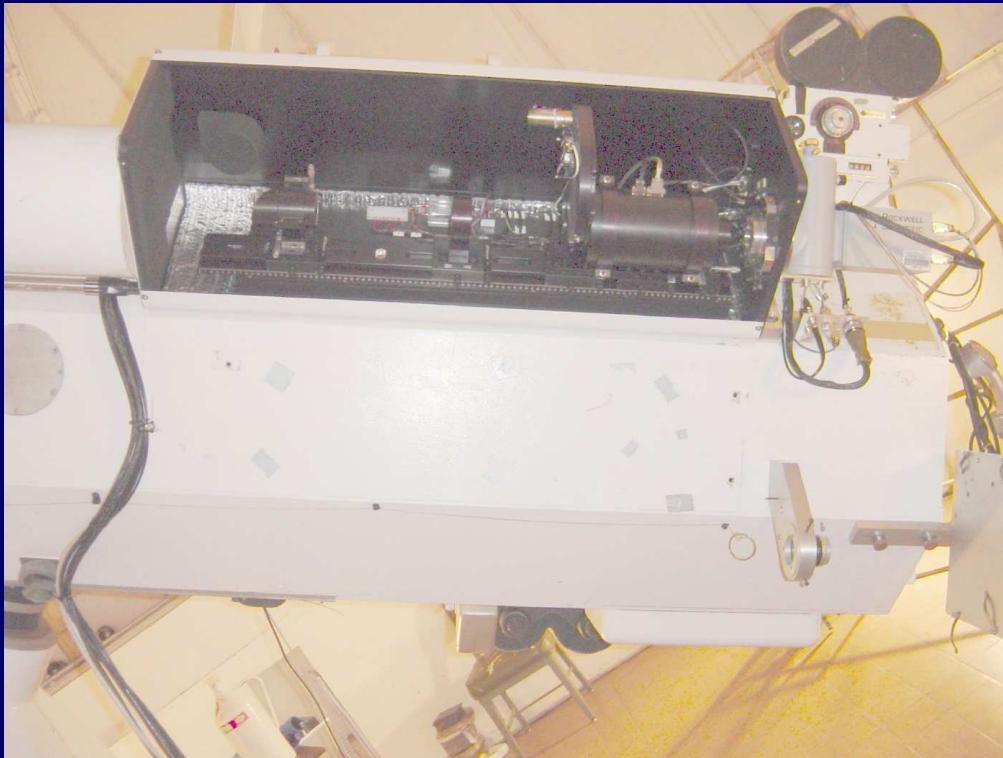
Multi-Channel Polarimeter for Coronal Magnetic Field Measurements.
