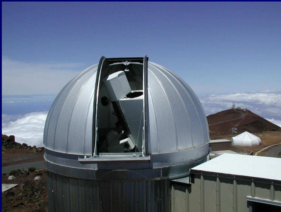
The SOLARC off-axis reflecting coronagraph. Gregorian, off-axis, “scatter free”.
